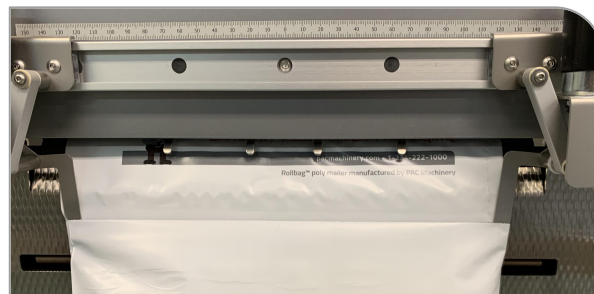
Seal flattener fingers go into the bag and stretch the top tight during sealing, to create a straight and clean final seal appearance
