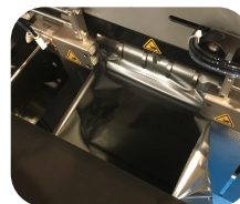
Easy load bag opener squares open and grips the bag
