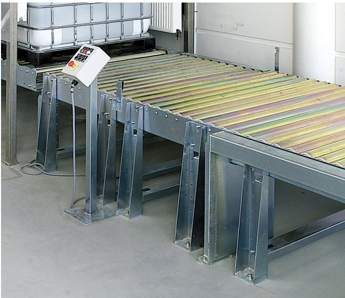
Driven pallet conveyor system at Coloplast in Denmark.
