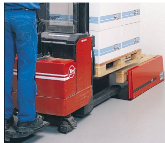
The pallet exchanger is easily adjusted for the specific pallet size by changing the distance between the two side modules. The modules are then bolted to the floor.
