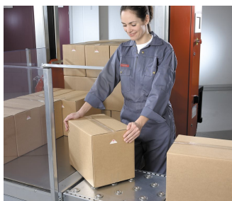
The ball table facilitates transfer to the stripper plate (accessory).
