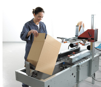
The front and rear flaps are folded towards the rail.
