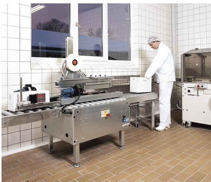
T-10 with stamp coder Various coding equipment is available for the T-10 series: side, top and bottom coders. (Kirk Food A/S)
