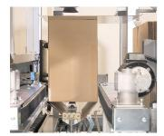
Efficient bottom flap folding and glue application.
